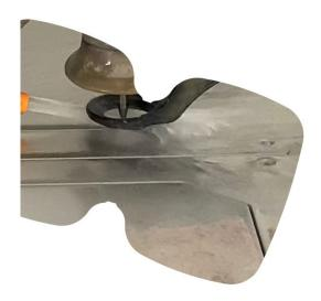
Minimal heat is added in the cutting process yielding no affects to the Rockwell hardness near the striking areas on the anvils.
